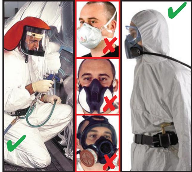
95 Half-mask BA (with constant airflow supply) conforming to BS EN 139:1995, or to Class LDM 2 of BS EN 12419:1999, has also proved to be effective and does not need to be removed to see the quality of the work. Half-mask BA should be face-fit tested. You may also find it beneficial to have a separate visor or goggles, to protect against paint splashes.
