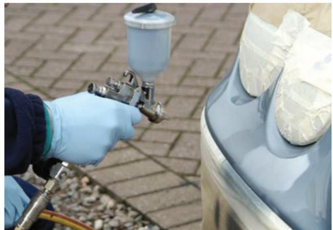
**Figure 19** SMART spraying with a mini-jet gun
